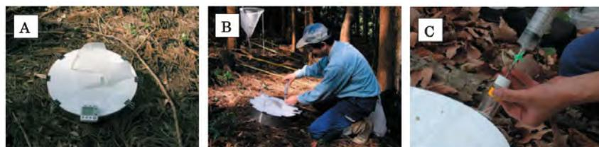
Figure T02-2 Measurement of greenhouse gas by flux method <sup>4)</sup>
