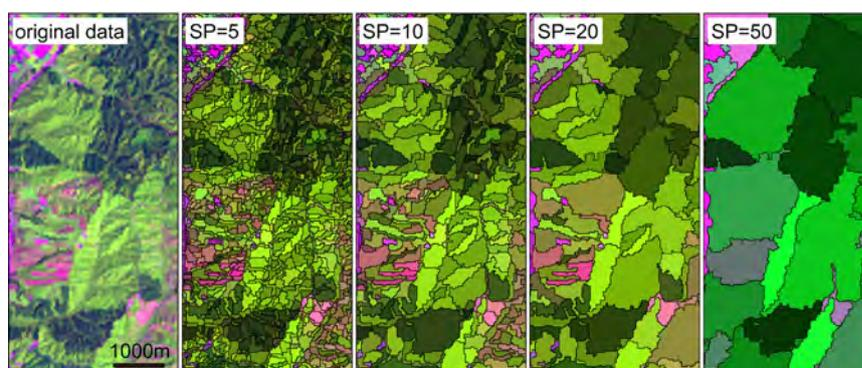
Figure T09-2 Results of segmentation with different scale parameters
