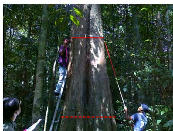
Fig T13-5 Measurement of diameter of tree with buttress root
