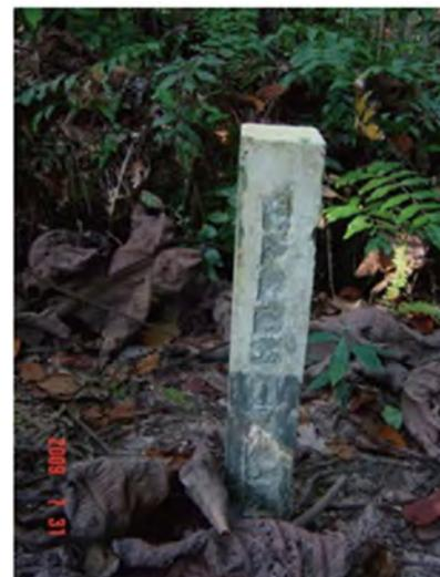
Figure T13-2 Example of stake which is resistant to disturbance (a concretestake)
